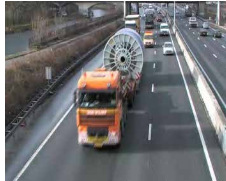
Figure 2: 400kV XLPE drums transported by truck
